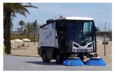
Madvac LS100 (Used by Montreal) Min Operating Width: 48 in Max Operating Width: 89 in Storage Capacity: 1.15 cubic yd
