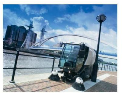
**Tennant Green Machines 636** Min Operating Width: 47 in Max Operating Width: 80 in Storage Capacity: 1.3 cubic yd
