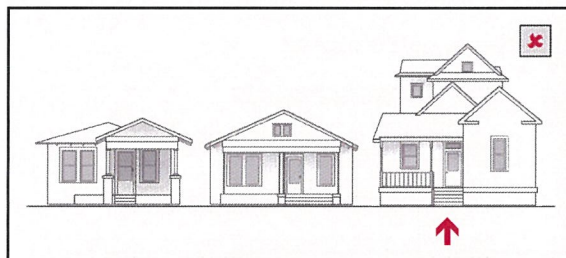
Incompatible addition; visually dominates original building
